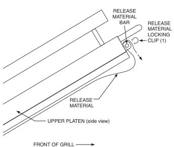
Check alignment and tightness of release material against upper platen.
